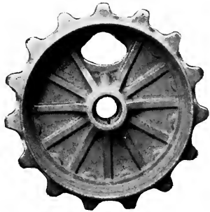
Fig. 25 Tractor Sprocket Wheel— Weight 115 pounds.
